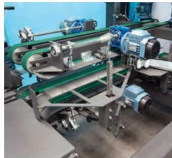
Automatic case closing with tape or hot melt. Motorised side guides. Auto adjustable.
