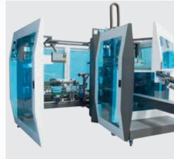
New ergonomic design. All machine parts are fully accessible by innovative sliding or opening guards. The collation module can easily be separated from the case packer module for change over and.
