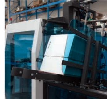
Blank picking system provided with motor.
