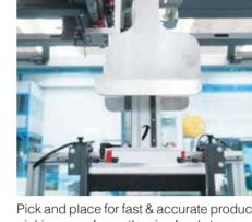
Pick and place for fast & accurate products picking up from the in feed transport conveyor and precise feeding of the carton with the configuration previously set.
