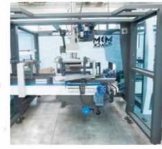
Completely accessibile and openable. Loading and cartoning stations are separable to allow operator entering for easy maintenance.
