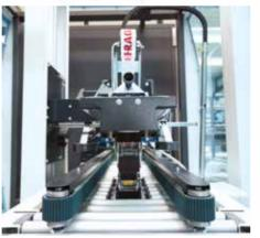
Out feed station with motorised driven belts adjustable for different carton sizes.
