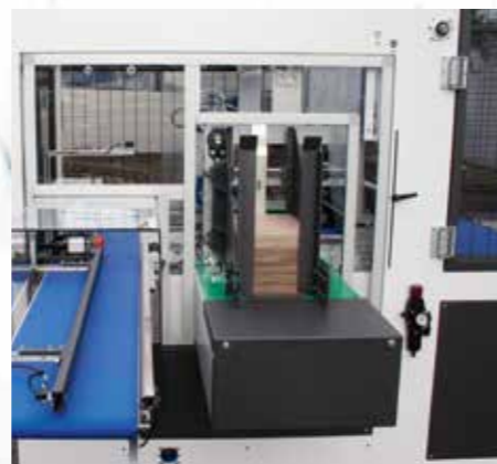
90° automatic grouping & feeding version. Different layout can be done for products feeding from left or from right.
