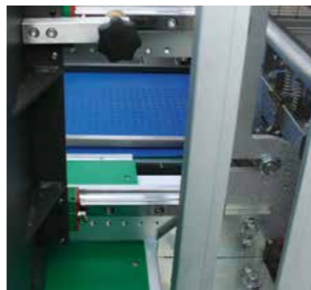
All movement on linear Hiwin guides.
